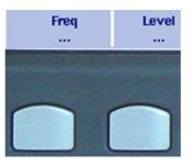
The horizontal softkeys provide access to the various menus. The name of the active menu is highlighted; the functions of a menu are offered on the vertical softkeys. Submenus are indicated with three dots ("..."); the menu softkey without the dots leads you one level up in the menu hierarchy.
