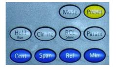
The function keys have specific functions which do not change. Therefore they are sometimes also referred to as "hardkeys" in contrast to the softkeys, whose functions change with the description given on the screen.
