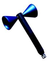
Biconical antennas are characterised by their dipole-like structure. The two reception lobes are highly symmetrical and provide the biconical antenna with two main reception directions with an opening angle of 120° each.
